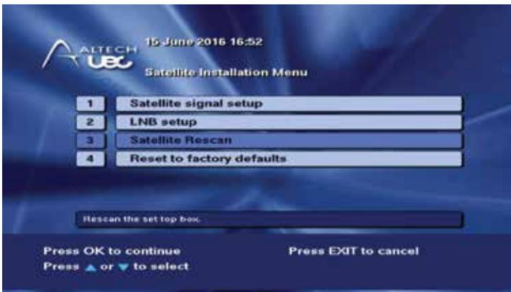
Press OK on “Satellite Rescan” to re-scan the set-top box with the new LNB settings.
